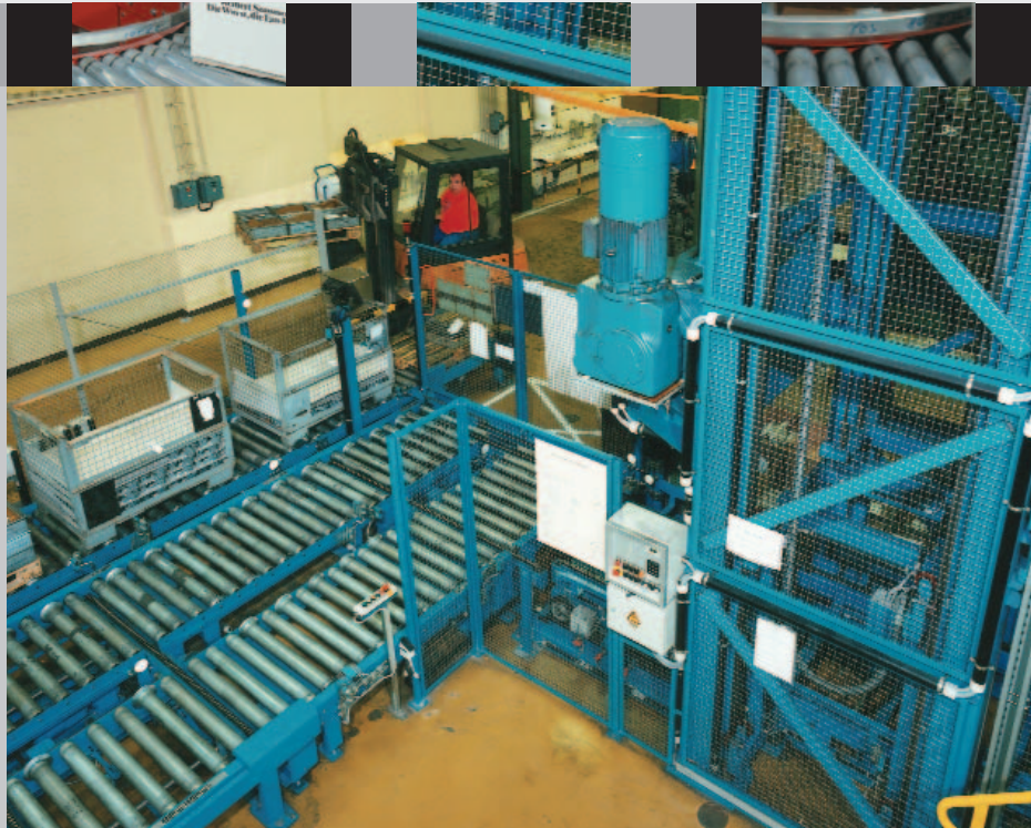
Pallet conveyor for euro, mesh, steel and special pallets
